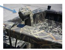
Squeeze the trigger and move the handle toward the engine to go into reverse. Move the handle towards the front of the boat to move forward.
