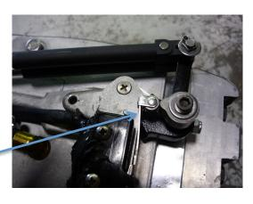
click in the switch when it turns on the start circuit. Test the shift and start procedure several times to ensure the engine starts. See the emergency starting procedure instruction sheet included with your quick start guide to bypass the start in gear protection if there is a micro switch failure in the field.
